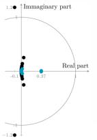
The blue (black) dots represent the eigenvalues for a stable (unstable) linear time-delay system. In the figure above, the time-invariant system is asymptotically stable if and only if all the infinitesimal generator eigenvalues are contained in the left-complex plane. In the figure on the left, the timeperiodic system is asymptotically stable if and only if the monodromy operator nonzero eigenvalues are strictly contained in the complex unit circle.
